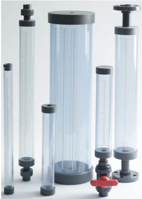
**Griffco** calibration cylinders are designed to enhance the performance of chemical feed systems by providing a verification of the flow rate of the chemical feed pump. Robust construction of clear PVC with an easy to read graduation in mL and gph. Available in three models: EZ-Clean, Vented, and Open Top; and in 15 sizes: 100 mL through 40,000 mL as detailed here.
