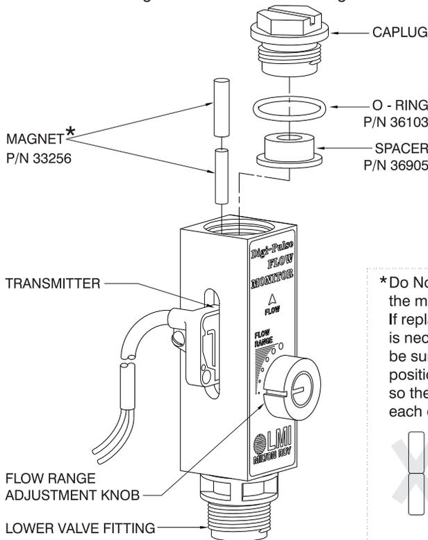
\*Do Not remove the magnets. If replacement is necessary, be sure to position them so they repel each other.
