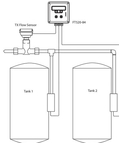
**Connections for Alternating Tanks**
